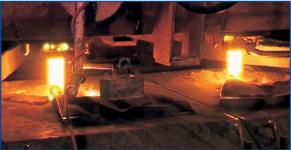
The steel is poured into moulds
