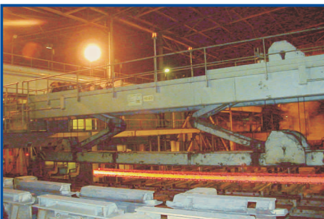
Transport of the Beam Blanks to the rolling mill
