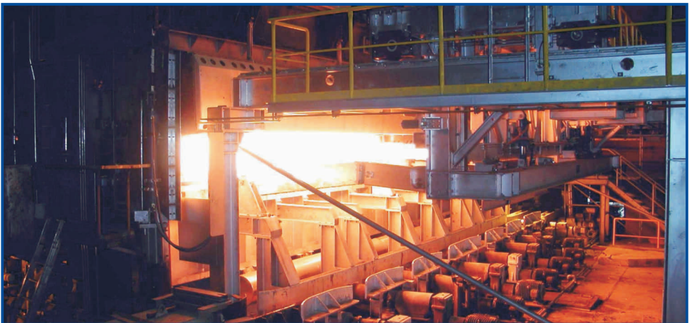
Exit pusher type furnace with discharging device
