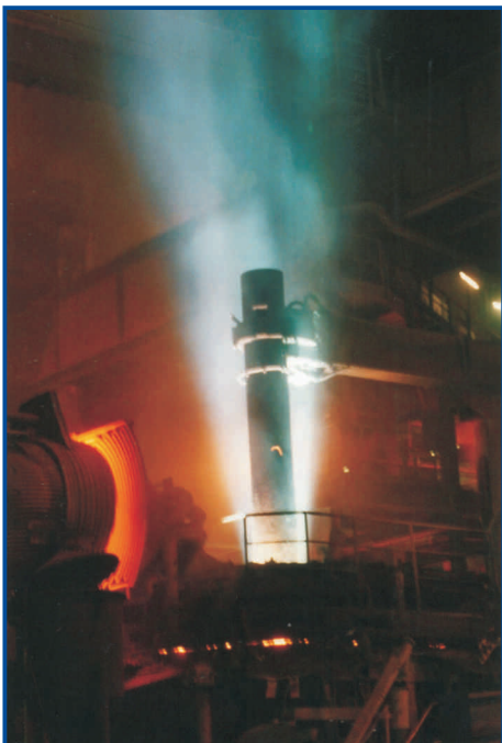
The DC electric arc furnace in operation
