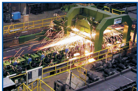
At the cold sawing unit the sections are cut for the customers
