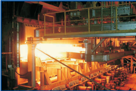
The pusher type furnace for the rolling mill runs on natural gas
